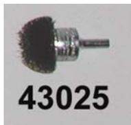
GMC brushes offered for this purpose are: Brass brush #43015 is for common tanks with large apertures, whereas #43035 is for small-necked models (hi-pressure steel and old 1/2"-NGT thread types). These brushes can be operated by hand or with an electric drill. #43025 is another drill brush especially suited for cleaning the O-ring groove in large-necked cylinders.
